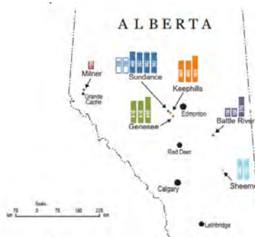
Figure 1. Coal-fired electricity generating units in Alberta (coloured bars denote unit size in MW) Data source: Milner Power, TransAlta, Aliso Power; map adapted from Natural Resources Canada
