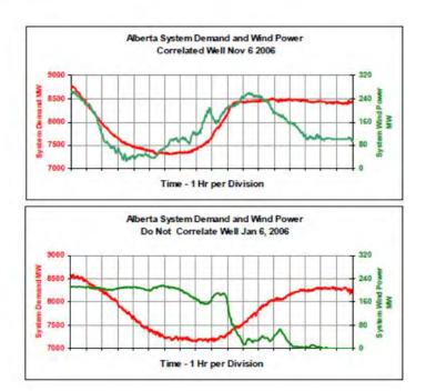
At the extreme, wind power may be at full capacity during light load periods just as other generating units approach their minimum stable operating levels. These studies also illustrated how ramping (20 minute to hours) of wind generation rather than intra-hour variability presented the greatest operational challenges.
