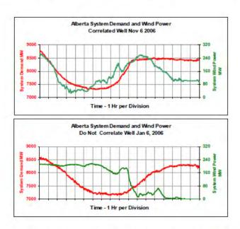
At the extreme, wind power may be at full capacity during light load periods just as other generating units approach their minimum stable operating levels. These studies also illustrated how ramping (20 minute to hours) of wind generation rather than intra-hour variability presented the greatest operational challenges.
