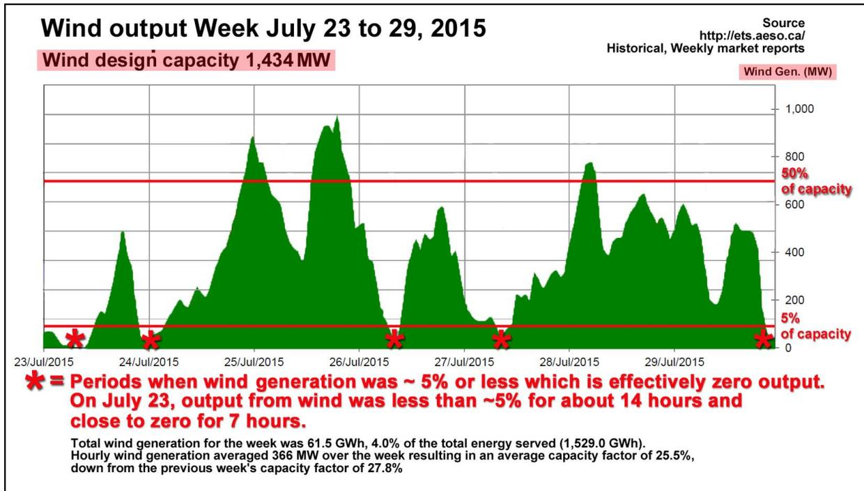
This week wind output was 25% of capacity, which is quite high, but the graph also shows how erratic wind output is. Two and three weeks before, output was a mere 13% of nameplate capacity. Wind output is at or near zero several times almost every week. Imagine attempting to run all parts of our society if we had to rely on wind. In winter, reliance on wind would be outright dangerous.
