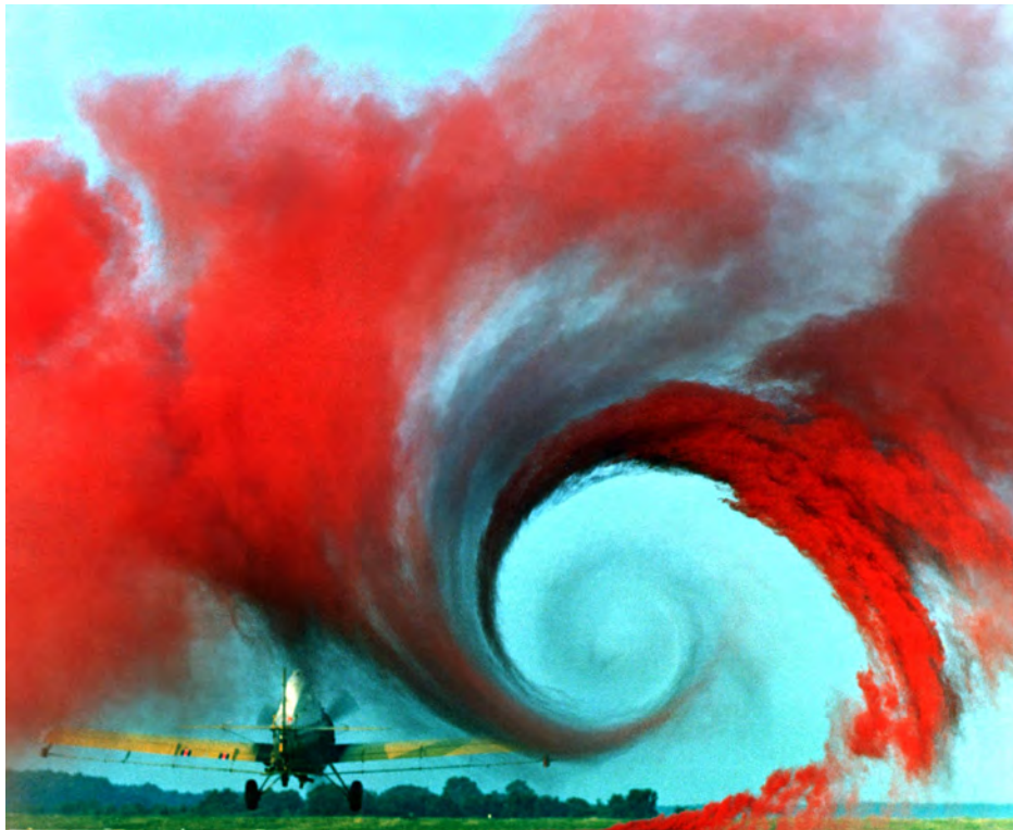
A visualization of air turbulence from the wing tip of an aircraft. Weather systems exhibit similar large and unpredictable turbulence and ‘chaos’ on vastly larger scales.
